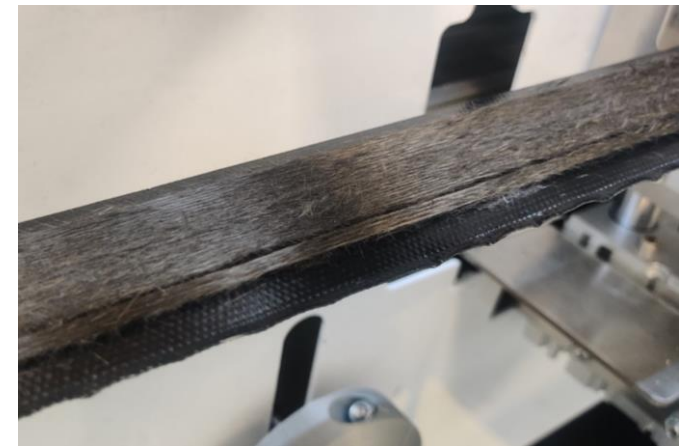
HiPerDiF highly aligned tape
