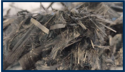
80 mm long pyrolyzed fibres, rCF(p)
