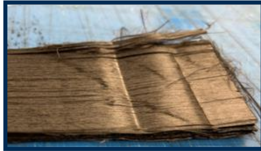
950 mm long steam-pyrolyzed fibres, rCF(s)
