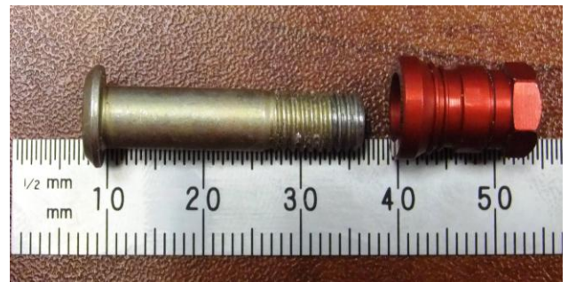
Fig. 3. Double shear bolt and collar
