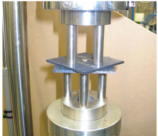
Fig. 4. Pull-through test set-up
