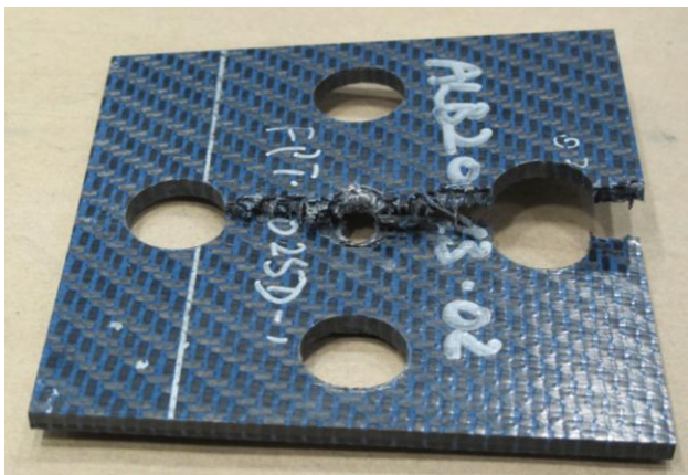
Fig 9. Typical flexural failure mode demonstrated in pull through testing
